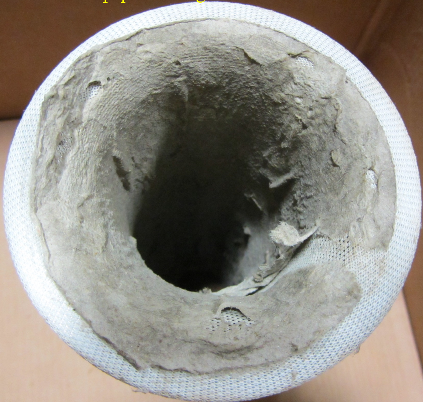
Toilet paper coating filter and 600 micron sock
