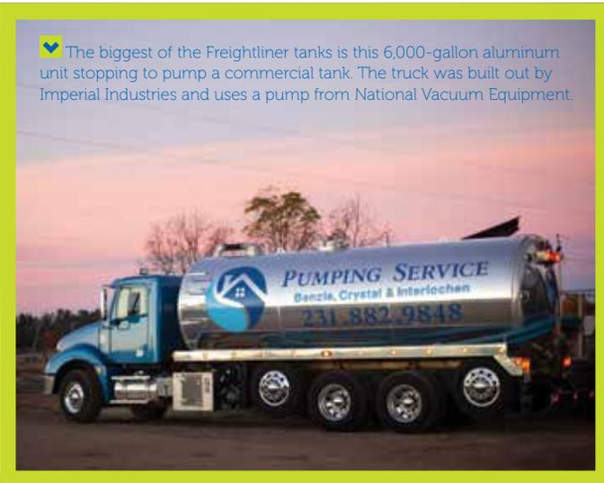
✔ The biggest of the Freightliner tanks is this 6,000-gallon aluminum unit stopping to pump a commercial tank. The truck was built out by Imperial Industries and uses a pump from National Vacuum Equipment.
